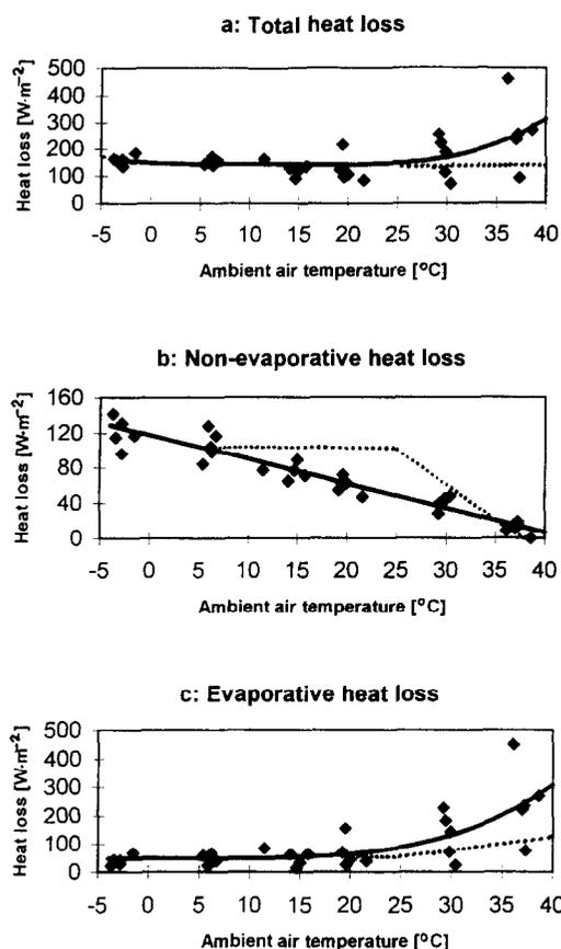
Fig. 1. The three diagrams show relationship between (a) total; (b) non-evaporative; and (c) evaporative heat loss and ambient air temperature. The dotted lines represent the theoretical model [according to a thermogram by Mount (1973)] and the solid lines and data points are results (Morgan *et al.*, 1997).
