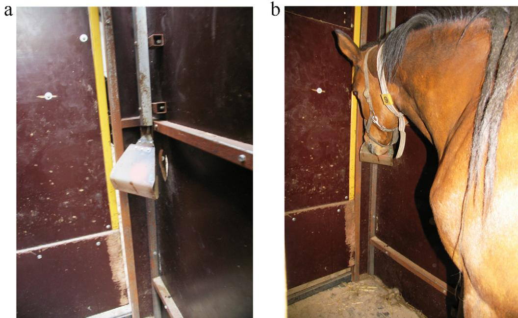
**Fig. 2.** Illustration of the operant panel (a) and a illustration of a horse pressing the operant panel (b).
